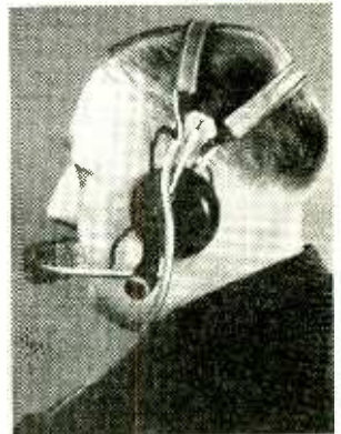
Headphone mounting for Lustraphone noise-cancelling microphone and (below) sensitivity/distance and polar characteristics at 1000 c/s.
